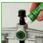
**Puller spindle maintenance:** The spindle must always be kept well lubricated. We recommend the use of KUKKO special sliding grease for pressure spindle (Art. No.: 699999), or KUKKO Bio Multi Oil (Art. No.: 699990). A tube of KUKKO special sliding grease for pressure spindle is free with every order of an original KUKKO puller.
