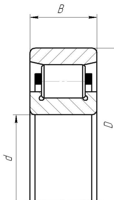
CYLINDRICAL ROLLER BEARINGS WITHOUT RIBS ON
