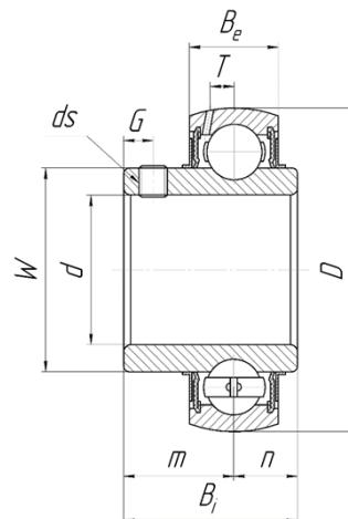
SPHERICAL BALL BEARING INSERTS
