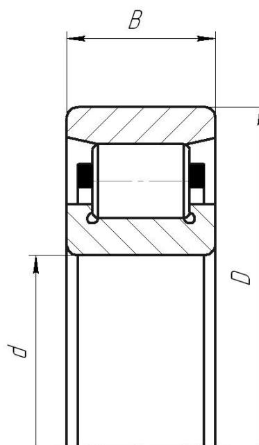
CYLINDRICAL ROLLER BEARINGS WITHOUT RIBS ON
