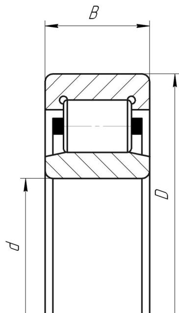
CYLINDRICAL ROLLER BEARINGS WITHOUT RIBS ON
