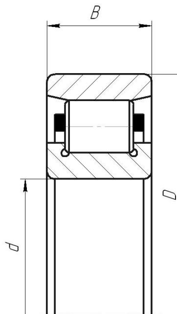
CYLINDRICAL ROLLER BEARINGS WITHOUT RIBS ON
