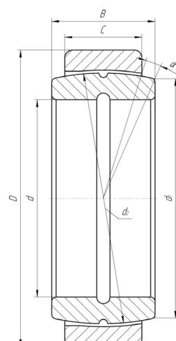
SPHERICAL PLAIN BEARINGS WITH LUBRICATION GROOVES AND HOLES IN THE INNER RING
