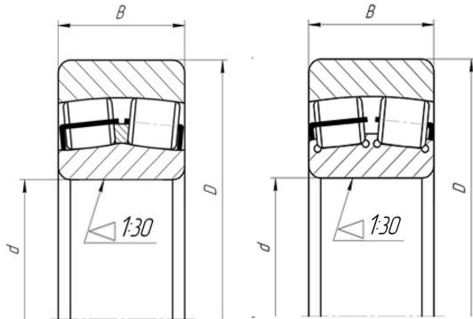
**SPHERICAL ROLLER BEARINGS WITH THE RIBLESS
