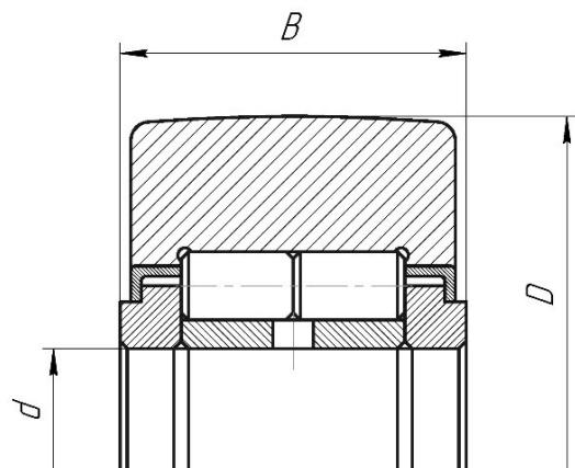
CYLINDRICAL ROLLER BEARING WITH SHORT CYLINDRICAL ROLLERS WITH TWO INTEGRAL RIBS ON THE INNER AND OUTER RINGS WITH A PROTRUDING INNER RING
