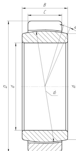
SPHERICAL PLAIN BEARINGS WITHOUT LUBRICATION
