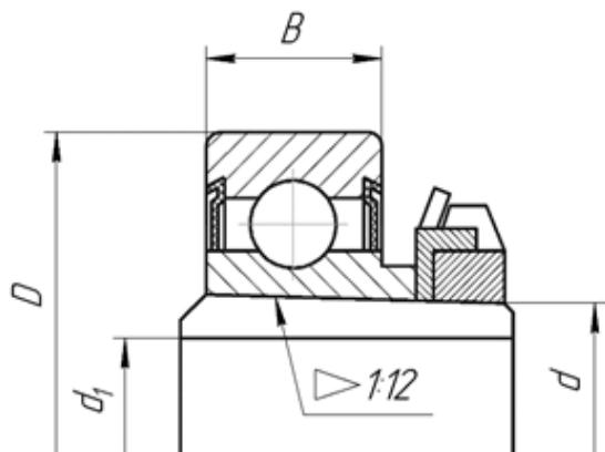
SINGLE ROW DEEP GROOVE BALL BEARINGS WITH A SEAL ON BOTH SIDES AND ADAPTER SLEEVE
