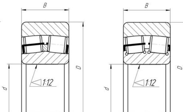
**ŁOŻYSKA BARYŁKOWE, DWURZĘDOWE, Z OTWOREM STOŻKOWYM NA PIERŚCIENIU WEWNĘTRZNYM,
