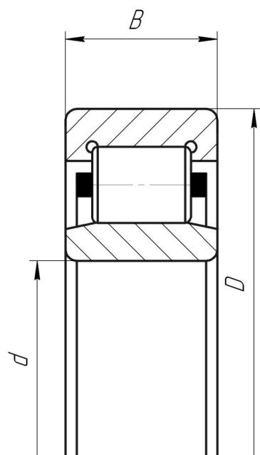
CYLINDRICAL ROLLER BEARINGS WITHOUT RIBS ON
