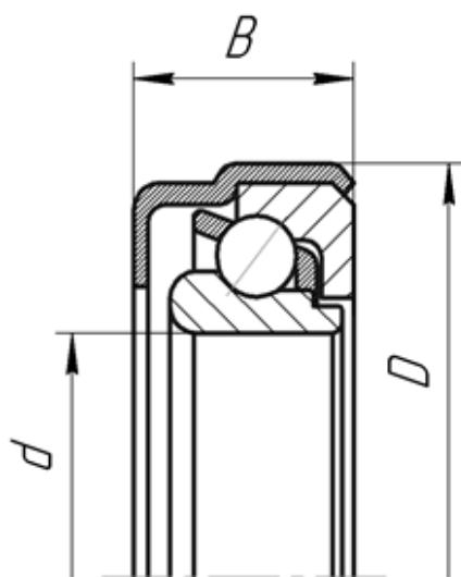
SPECIALLY DESIGNED SINGLE ROW ANGULAR CONTACT
