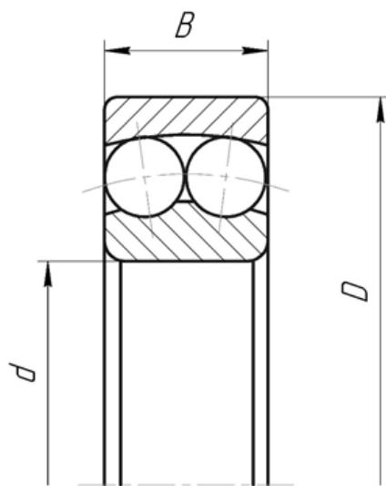
DOUBLE ROW SPHERICAL BALL BEARINGS WITH
