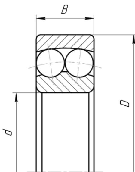
DOUBLE ROW SPHERICAL BALL BEARINGS WITH
