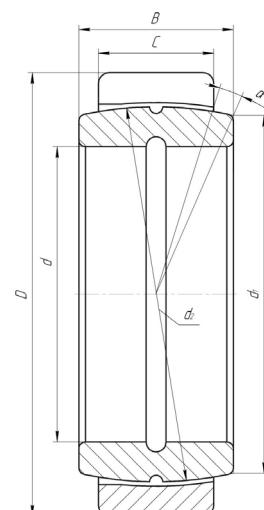
SPHERICAL PLAIN BEARINGS WITH LUBRICATION GROOVES AND HOLES IN THE INNER RING AND WITH THE OUTER RING FRACTURED AT ONE POINT
