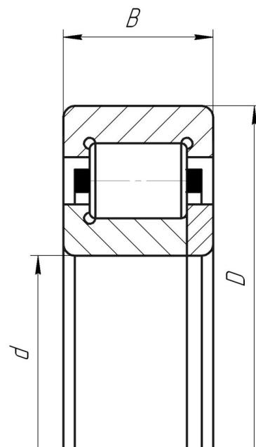
CYLINDRICAL ROLLER BEARINGS WITH TWO INTEGRAL RIBS ON THE OUTER RING, ONE INTEGRAL RIB AND ONE LOOSE RIB ON THE INNER RING
