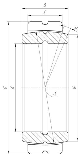
SPHERICAL PLAIN BEARINGS WITH LUBRICATION GROOVES AND HOLES IN BOTH RINGS AND WITH THE OUTER RING FRACTURED AT TWO POINTS
